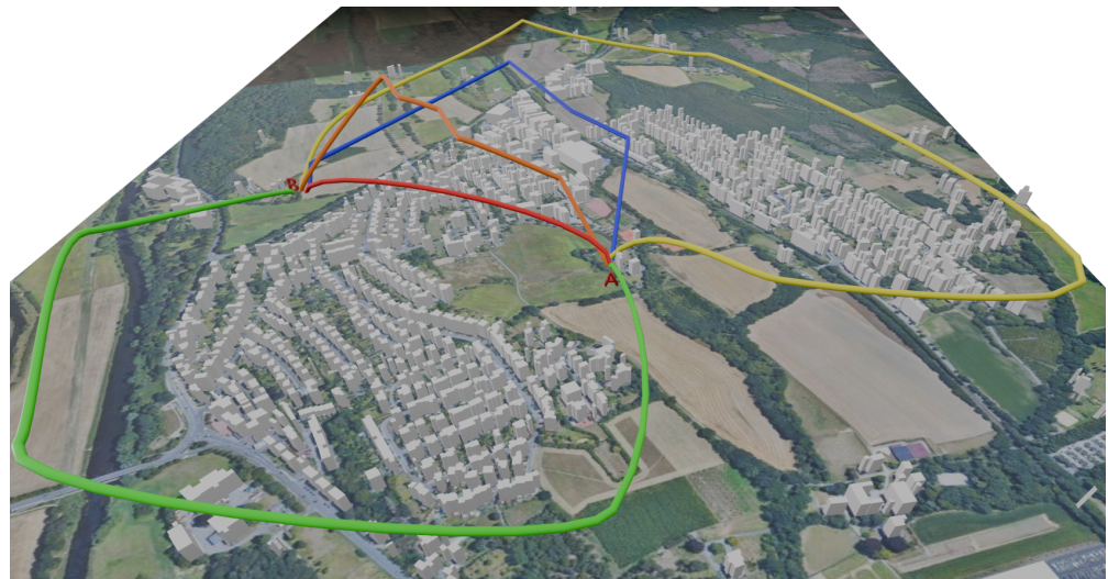
Figure 21. Five distinct route suggestions are proposed for a delivery drone, each differing in safety levels and distance to the target. The starting location is denoted by A, while B represents the target.
