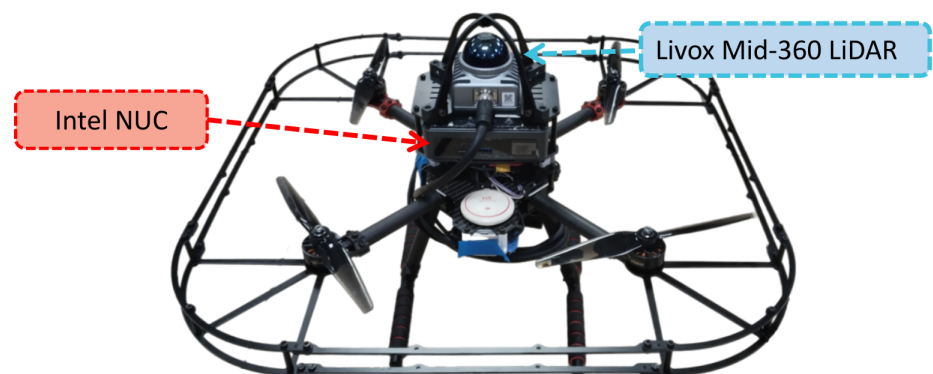
Figure 13. The flying platform used in real-world experiments: a quadrotor drone equipped with an Intel NUC and a Livox Mid-360 LiDAR sensor.
