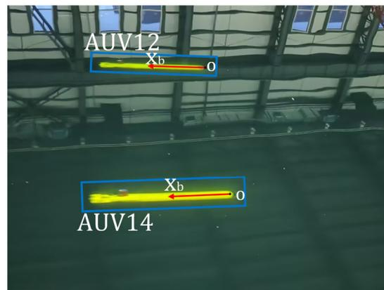
**Figure 14.** Experimental setup illustration. AUV12 and AUV14 during the coordinated navigation localization experiment, with each AUV’s coordinate axis ( $X_b$ ) and origin ( $O$ ) marked as reference points.
