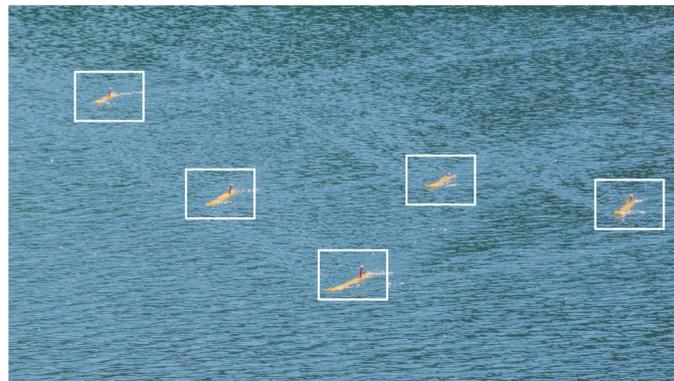
**Figure 1.** Swarm navigation of “TS-MINI” AUVs. Five TS-MINI AUVs, developed by the Shenyang Institute of Automation, Chinese Academy of Sciences, are performing a surface mission.
