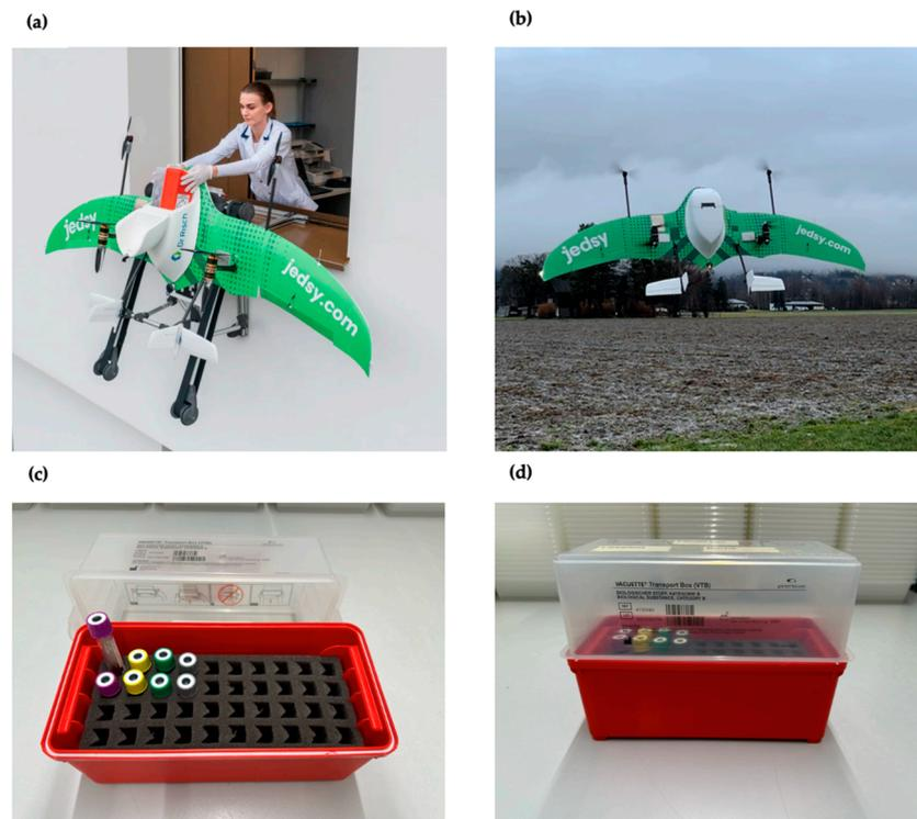
**Figure 1.** Images of the Uncrewed Aerial Vehicle (UAV) used for medical transport and the blood sample containers employed in the study. (a) Drone used for the tests. (b) Drone in hovering mode. (c) open safety box. (d) safety box to transport the blood samples.
