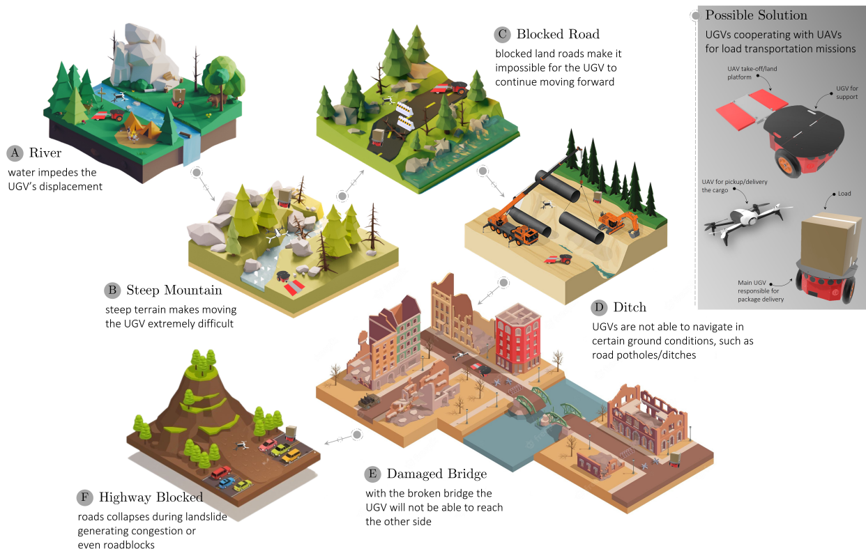
Figure 1. UGV load transportation limitations due to specific environment constraints. A possible solution for delivery packets in long-distance missions is the cooperation between UAV and UGVs in the mission planning step.
