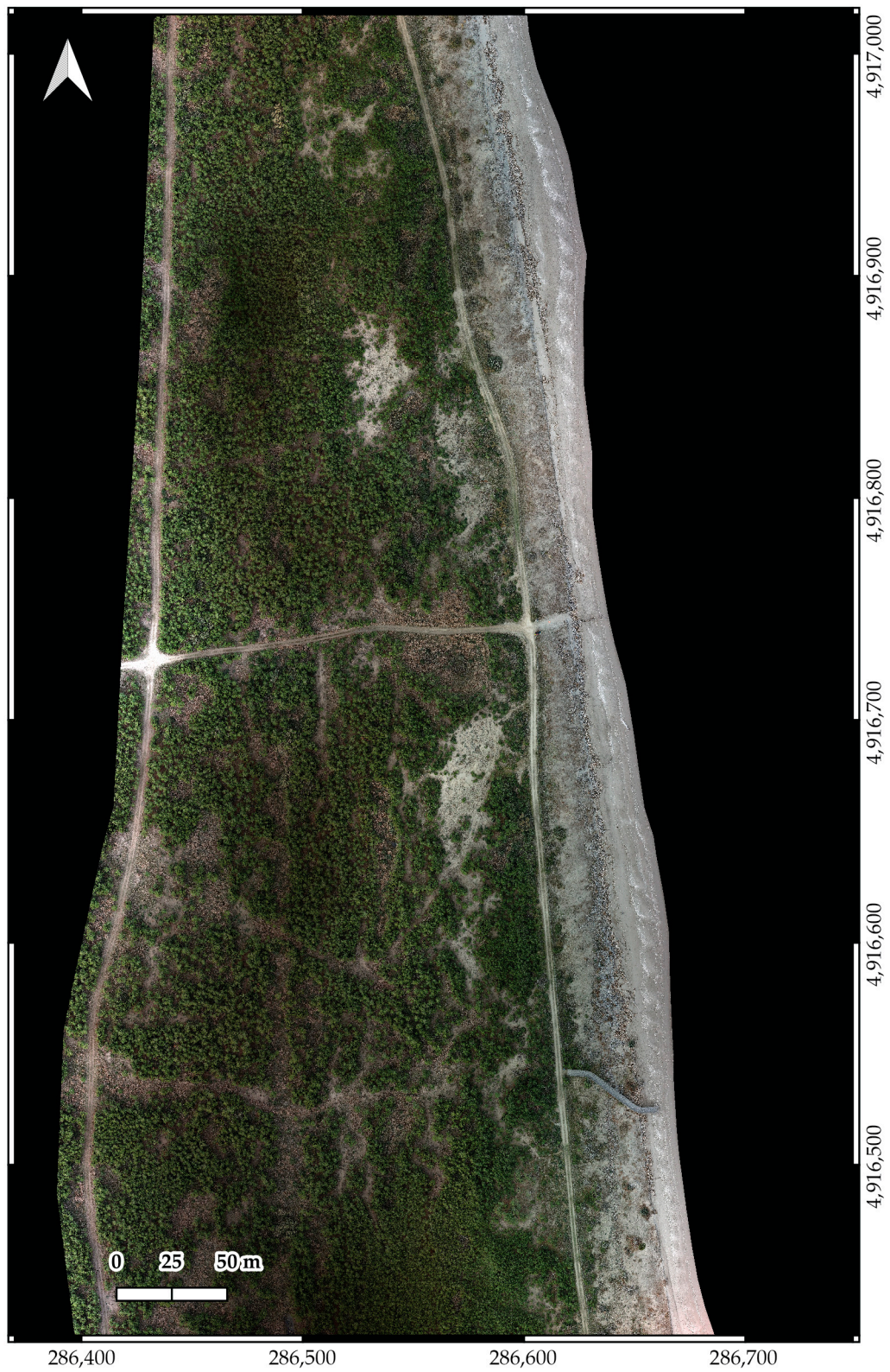
Figure S2. The orthomosaic of the scene, map coordinate reference system RDN2008/UTM33, meter unit. Output with a GSD (Ground Sampling Distance) of 6 mm and subsampled at a resolution of 10 cm.
