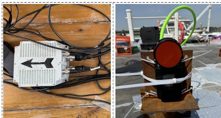
**Figure 4.** The device on the left is the SINS, and the device on the right is the DVL device.
