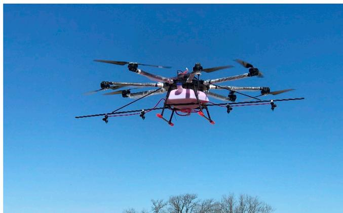
**Figure 1.** The V8A Pro aircraft with a 20 L payload capacity, eight (8) rotors, and four (4) spray nozzles on a boom used for this study. The nozzles were 18" (45.7 cm) and 32" (81.3 cm) from the center of the aircraft for inboard and outboard nozzles, respectively.
