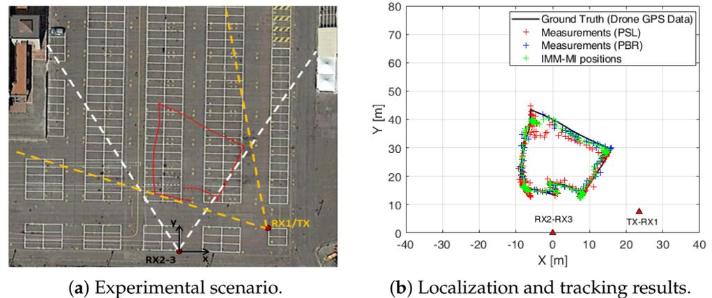
**Figure 8.** Experimental scenario and results for passive radar and RF joint detection in [83]. The left subfigure shows the experimental scenario setup, while the right subfigure presents the localization and tracking results of the drone on the  $x$ - $y$  plane using sensor fusion.
