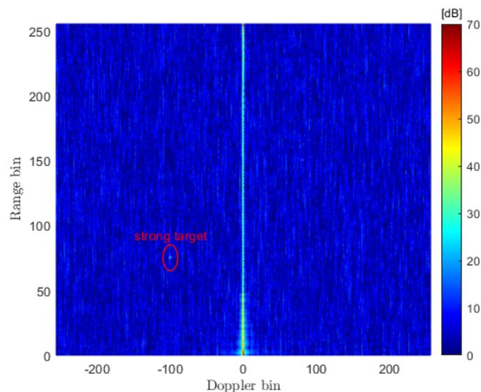
**Figure 4.** The RD map redrawn with RpF from Figure 3, effectively reducing the ambiguity floor and eliminating the “ghost peaks”, revealing a strong target.
