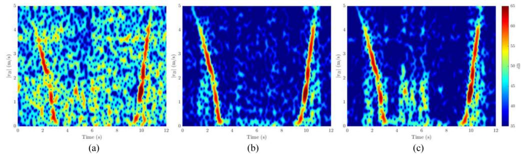
**Figure 7.** The results of using WiFi signal-based passive detection of UAVs without reference signals, as presented in [91], are shown in the figure. (a) The initial detection scenario with high background noise, (b) The application of traditional suppression algorithms using a reconstructed reference signal, and (c) The results achieved using the reference-free detection algorithm.
