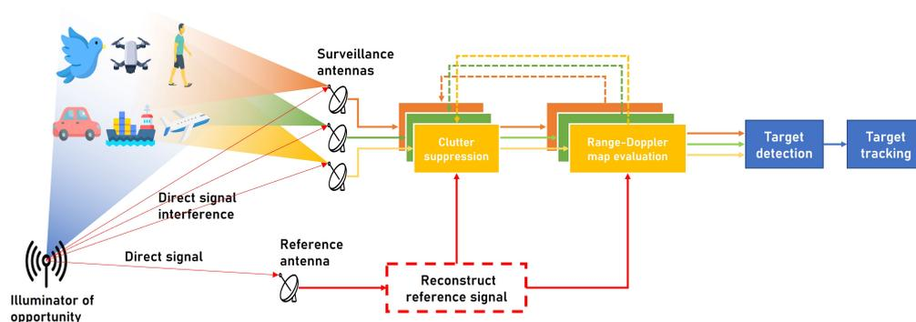
**Figure 2.** The typical signal processing flow of a passive radar system.
