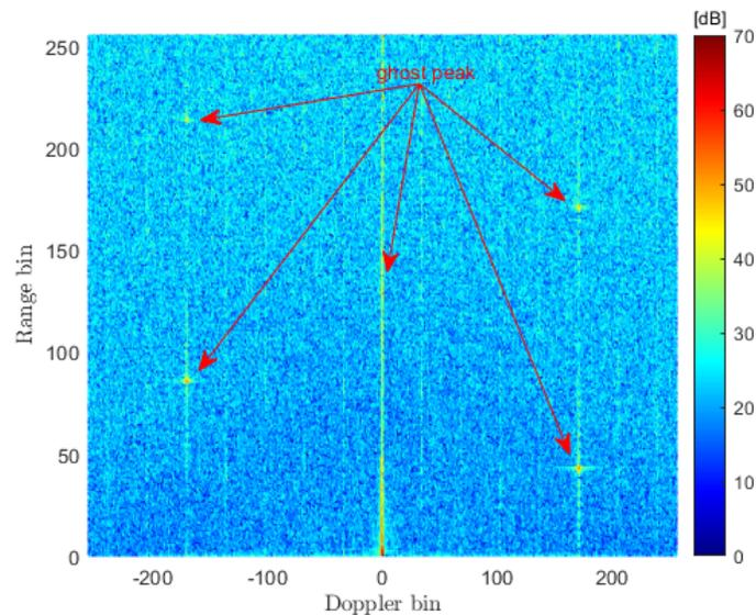
**Figure 3.** The RD map of the classic scenario for near-range UAV detection using passive radar simulation with MF, showing a high ambiguity floor and cyclically distributed “ghost peaks”.
