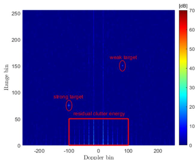
**Figure 5.** The RD map after applying the ECA-B Algorithm with RpF, effectively suppressing the ambiguity floor and revealing a weak target but showing a non-ideal structure in the RD map.
