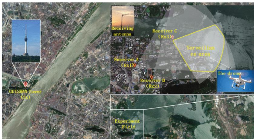
**Figure 6.** The drone detection experiment trial in [87] uses three single-antenna receivers at different positions. Their combined coverage detects the UAV, and the highest quality reference signal is shared for signal processing, followed by trajectory fusion.
