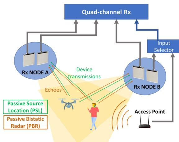
**Figure 9.** Sketch of a system setup implementing the PBR and PSL approaches [83].
