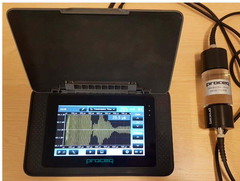
Figure 5. Calibration of the transducers before testing.
