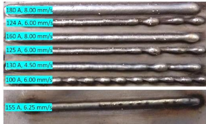
Figure 7. Bead-on-plate depositions (one layer) from the experiments carried out while determining the workable current range.
