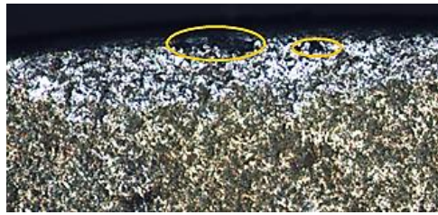
Figure 13. Slight tool wear observed when finish milling the workpiece built with the SSR of 67^\circ with v_c = 30 m/min, f = 0.1 mm/tooth/rev when milling in the XZ plane.
