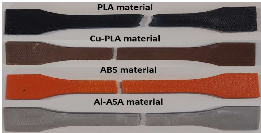
Figure 11. Fractured samples from the four materials.
