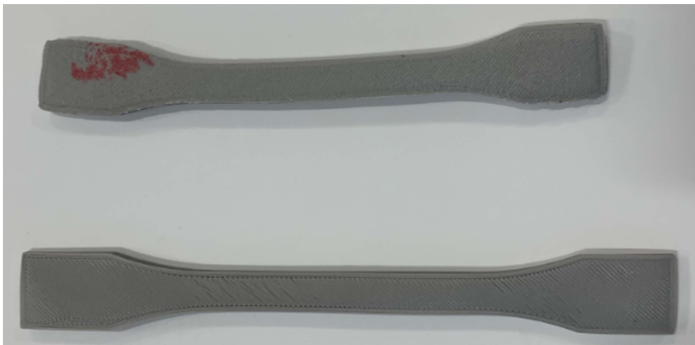
Figure 8. Significant deformation of Al-ASA at high annealing temperatures.
