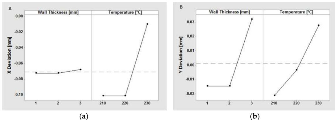
Figure 4. Plot of means for dimensional deviation for (a) the X dimension and (b) the Y dimension.
