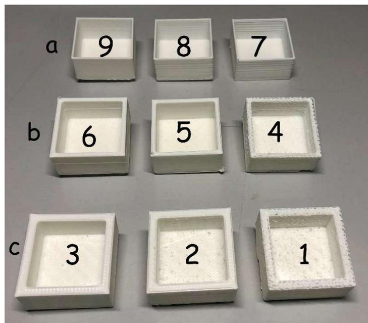
**Figure 2.** The nine printed items. From left to right: (a) First row (1 mm wall): Models 9 (230 °C), 8 (220 °C), and 7 (210 °C), (b) Second row (2 mm wall): Models 6 (230 °C), 5 (220 °C), and 4 (210 °C), (c) Third row (3 mm wall): Models 3 (230 °C), 2 (220 °C), and 1 (210 °C).
