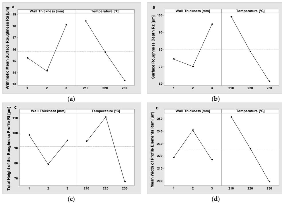
**Figure 5.** Plot of means for surface roughness parameters: (a) arithmetic mean surface roughness Ra, (b) surface roughness depth Rz, (c) total height of the surface roughness profile Rt, and (d) mean width of profile elements Rsm.
