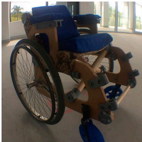
Figure 4. An open source wheelchair called the HU-GO.
