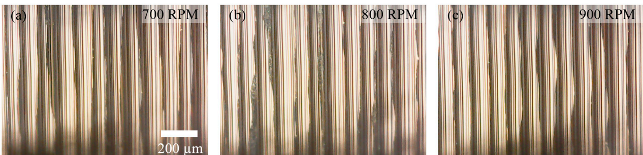
Figure 8. Microscope image of machined surface: (a) 700 rpm, (b) 800 rpm, and (c) 900 rpm.
