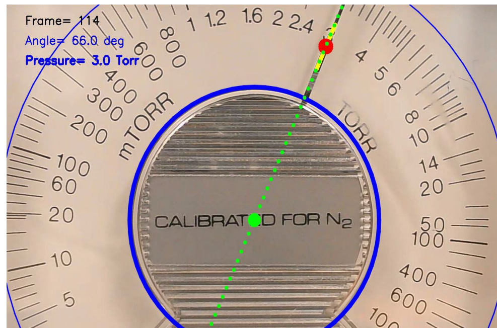
Figure 5. Sample frame from computer vision-based gauge reading system [38] (blue—dial circumference detected with Hough circle transform; yellow—gauge arrow pointer detected with grayscale threshold; red—middle part of the arrow pointer; green—direction to the arrow pointer according to the calculated angle of inclination).
