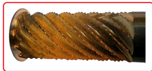
Figure 6. Accumulation of yellow powder on the CZ10 cutting tool.
