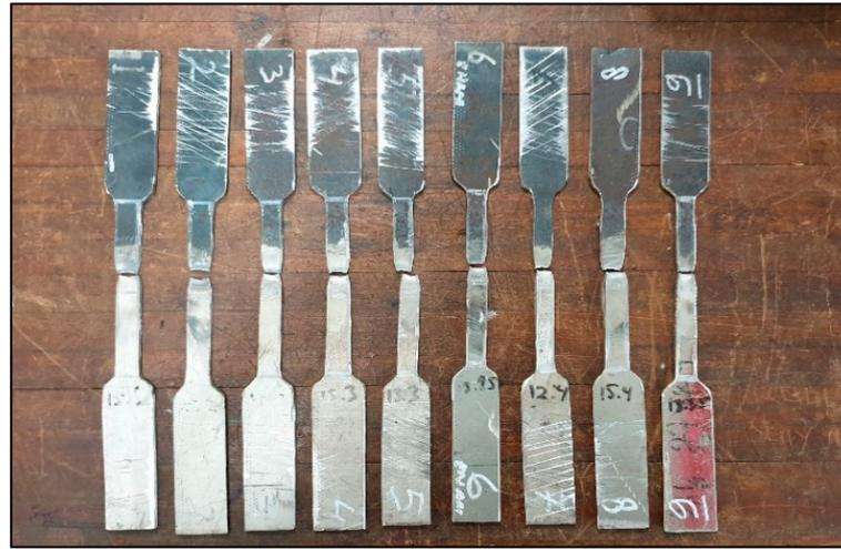
Figure 4. Tensile test samples of SS316 and low-carbon steel.
