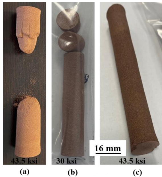
Figure 8. Consolidated CIPed bars, (a) as-received pure Cu at 303 MPa, (b) cryo-milled Cu at 207 MPa, and (c) cryo-milled Cu at 303 MPa.
