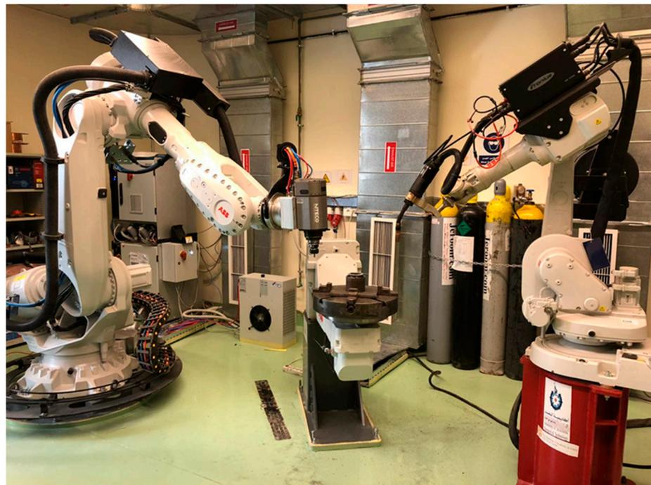
**Figure 1.** The additive/subtractive robotic-controlled manufacturing system, AMCL [20].
