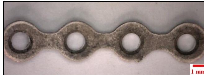
Figure 17. Miniplate product from microforming process.
