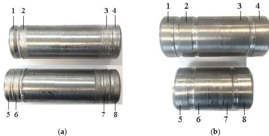
Figure 3. Machined workpieces made of different materials during cup cutter pre-processing: (a) bars \varnothing 50 mm of steel 45; (b) thick-walled pipes \varnothing 72 mm of steel 20X; 1— n_{sp} = 40 rpm (revolution per minute); 2— n_{sp} = 80 rpm; 3— n_{sp} = 20 rpm; 4— n_{sp} = 12 rpm; 5— \tau_d = 4 min; 6— \tau_d = 3 min; 7— \tau_d = 2 min; 8— \tau_d = 1 min.
