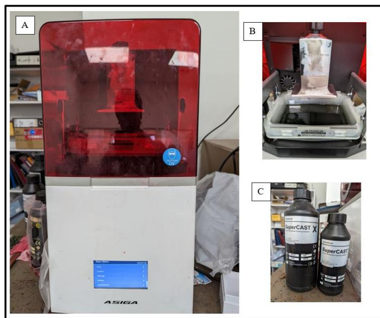
**Figure 7.** (A) Asiga MAX DLP printer (printing resolution: 62  $\mu\text{m}$ ). It uses a 385 nm (high-power UV LED) or 405 nm wavelength to cure the resin. (B) Inside the build chamber of the Asiga MAX printer, which shows the build tray full of resin ready to print. (C) Asiga SuperCAST X resin used for 3D model manufacture.
