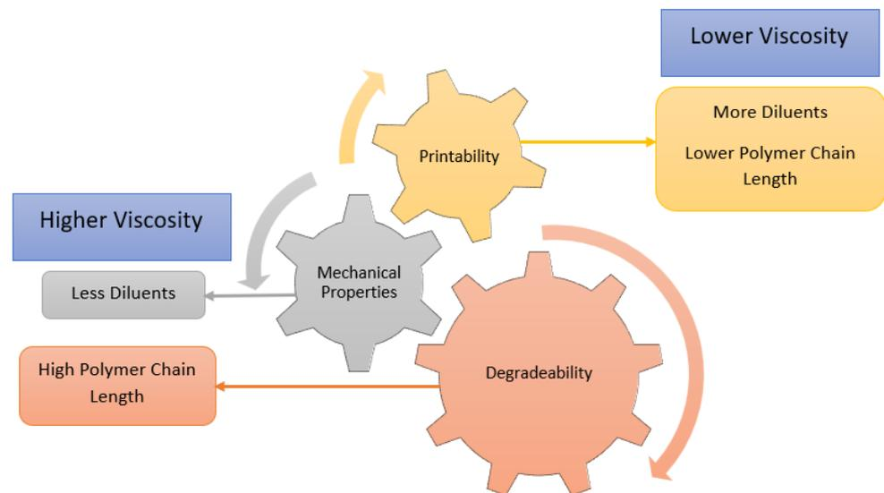
**Figure 3.** Relationship between resin viscosity, printability, mechanical properties and degradability [16].
