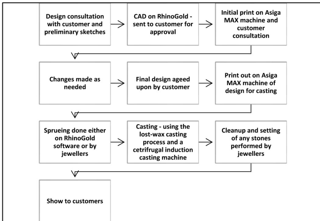
**Figure 8.** Sinclairs Jewellers process for creating personalised customer jewellery using AM. Design costs were greatly reduced due to the ease of producing life-like renders on RhinoGold, which also made design changes quicker due to the built-in features in the CAD programme. Jewellers are required for the clean-up and stone-setting phases.
