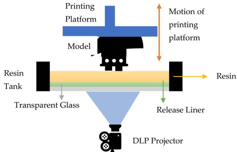
Figure 5. Schematic diagram and working procedure of a DLP print [31].
