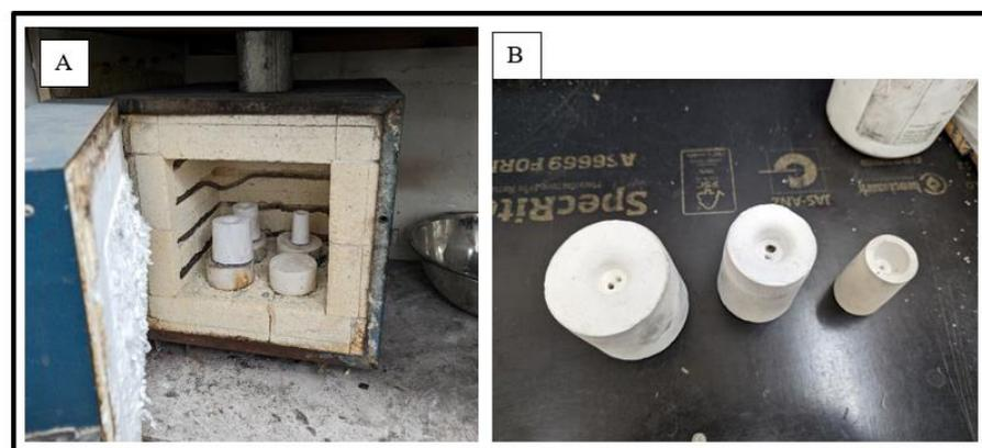
**Figure 9.** (A,B) Phosphate investment casts in the kiln after burnout. Asiga resins have a burnout schedule of 149 °C for 2 h, 371 °C for 2 h and 482 °C for 2 h, and then remain at 750 °C for 4 h. Then moulds are reduced to the cast temperature for 2 h and get ready to go to a centrifugal induction casting machine.
