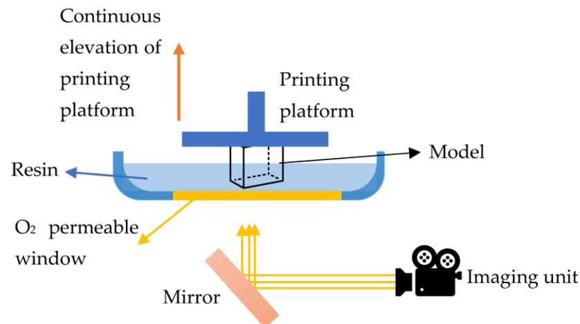
Figure 6. CLIP process shows layerless printing and the architecture of a CLIP printer [14].
