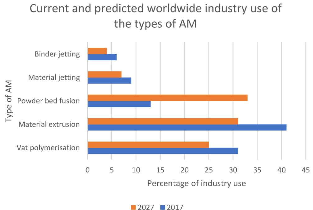
**Figure 1.** Percentage of revenue earned in the professional industry shows material extrusion such as fused filament fabrication (FFF) and fused deposition modelling (FDM) falling behind powder bed fusion (PBF). Vat polymerisation (VP) continues to fall in popularity due to a lack of diverse material availability and post-processing requirements [7–9].
