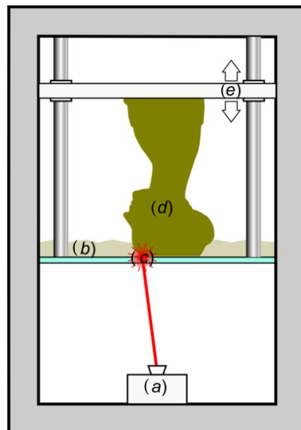
**Figure 4.** Schematic diagram of a SLA process. (a) laser or UV light device; (b) resin reservoir that has a clear film on the bottom to allow the light emitting device to cure the resin; (c) light emitting device curing the thin film of resin between the bottom of the resin reservoir and the solidified part of the 3D build; (d) the solidified part of the 3D build being lifted by the build platform; and (e) the printing platform. Paolo Cignoni, CC BY-SA 4.0.
