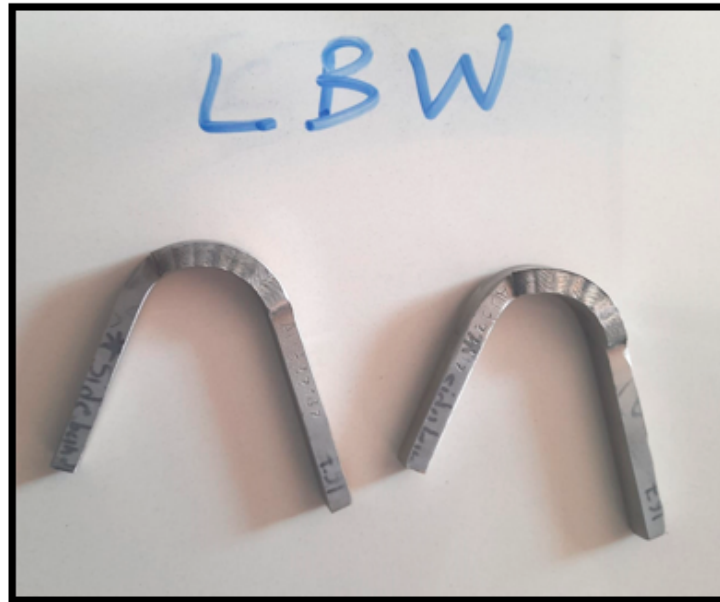
Figure 6. Hastelloy weld overlay bend test using LBW.
