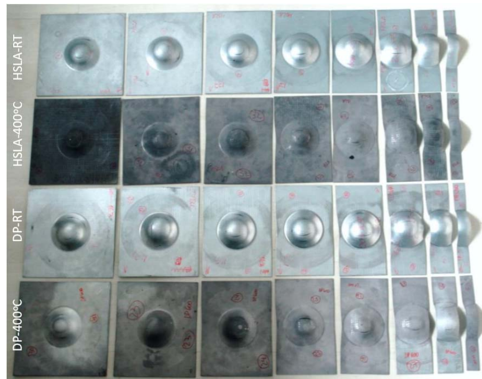
Figure 11. HSLA 350/440 and DP 350/600 experimental deformed sample at room temperature and 400 °C to determine FLC.
