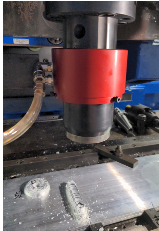
Figure 4. Tool holder with cooling collar (red), mounted die (silver), and fixturing. Background: linear and doughnut-shaped test extrusions.
