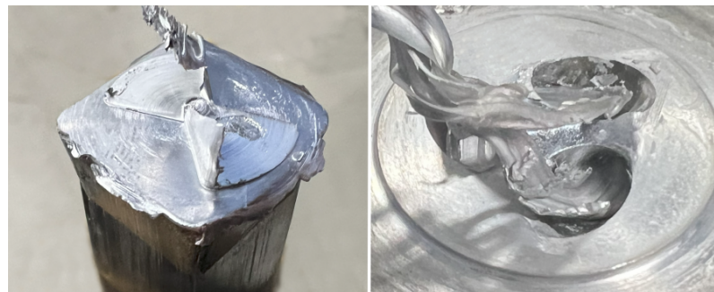
Figure 6. Ribbon formation (extrudate), as generated by two different die designs: bow-tie # 1 (left, end of the rod with visible bulging) and 45° tri-hole # 4 (right, still within a die).
