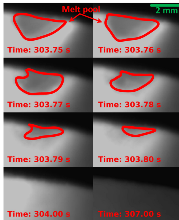
Figure 5. The progression of melt pool solidification after the laser was turned off. Note: t = 303.75 s corresponds to the moment at which the laser was turned off.
