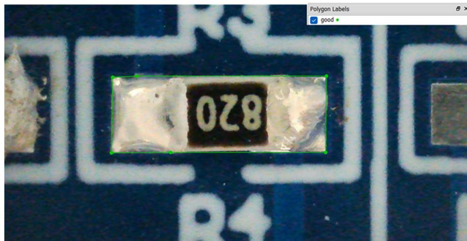
Figure 9. Correct positioning of the component (1)—good label.
