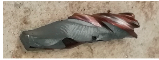
Figure 4. Broken tool at 3% emulsion concentration.
