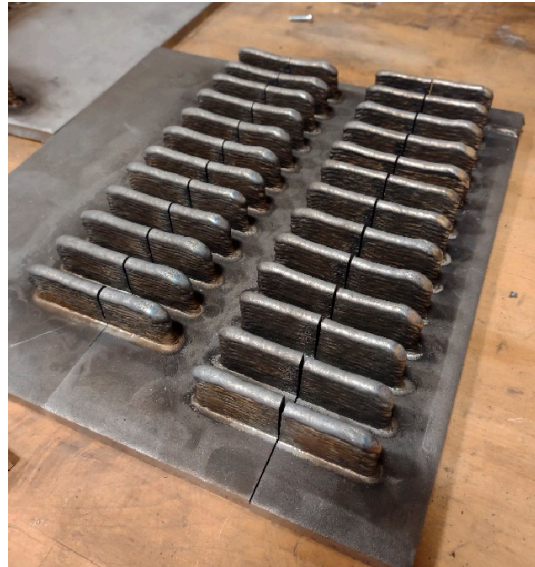
Figure 2. The 20-layer 80 mm single tracks deposited using Inconel 718 wire on a Gefertec Arc605.
