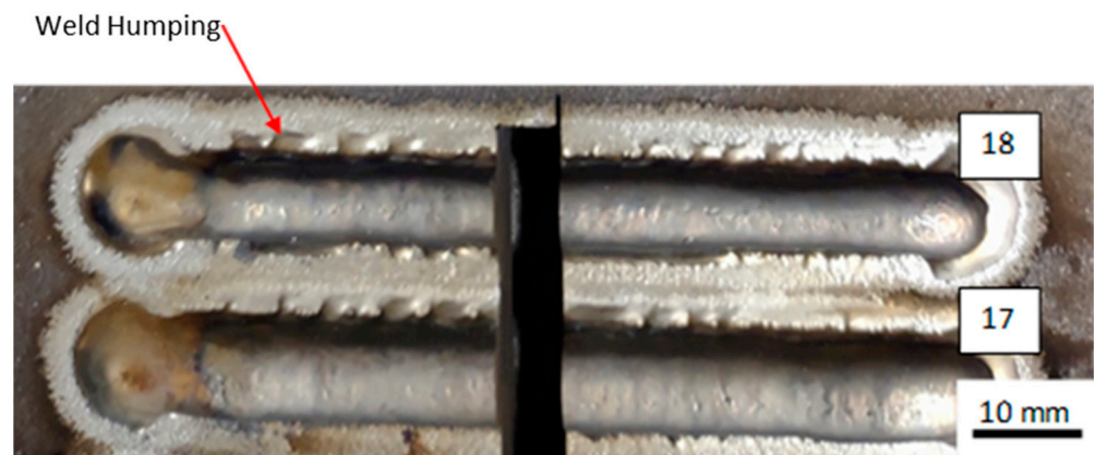
Figure 7. Specimen 17 and 18 from Table 1 showing humping of the weld (red arrow).
