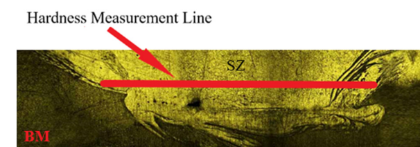
Figure 4. Schematic line depicting the path for microhardness measurements across the cross-section of processed samples.
