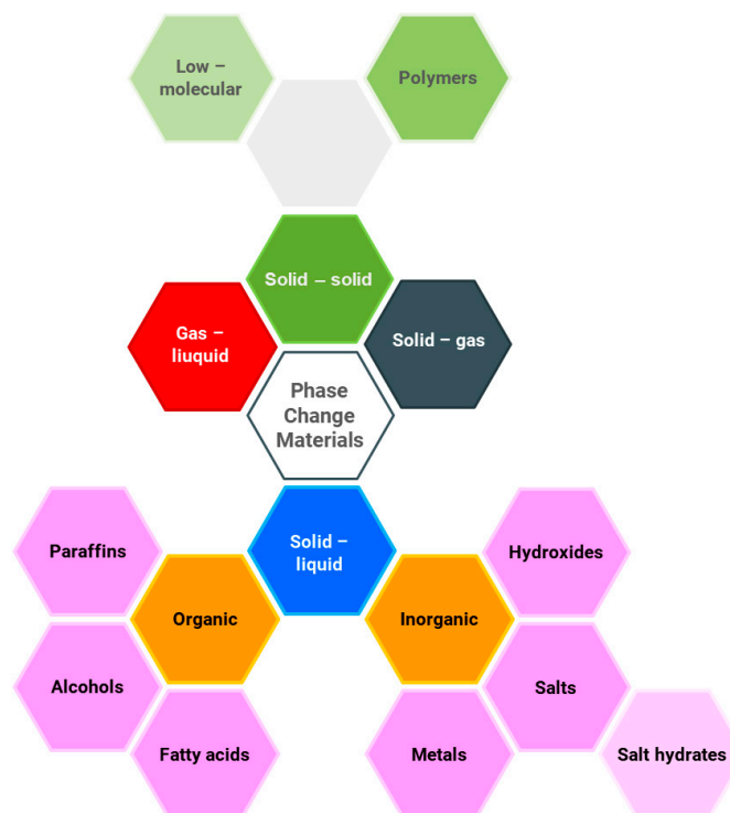
Figure 1. Classification of phase change materials (PCMs), based on [7].
