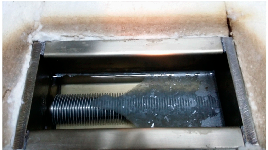
Figure 7. Heat storage unit with partially melted PCM.
