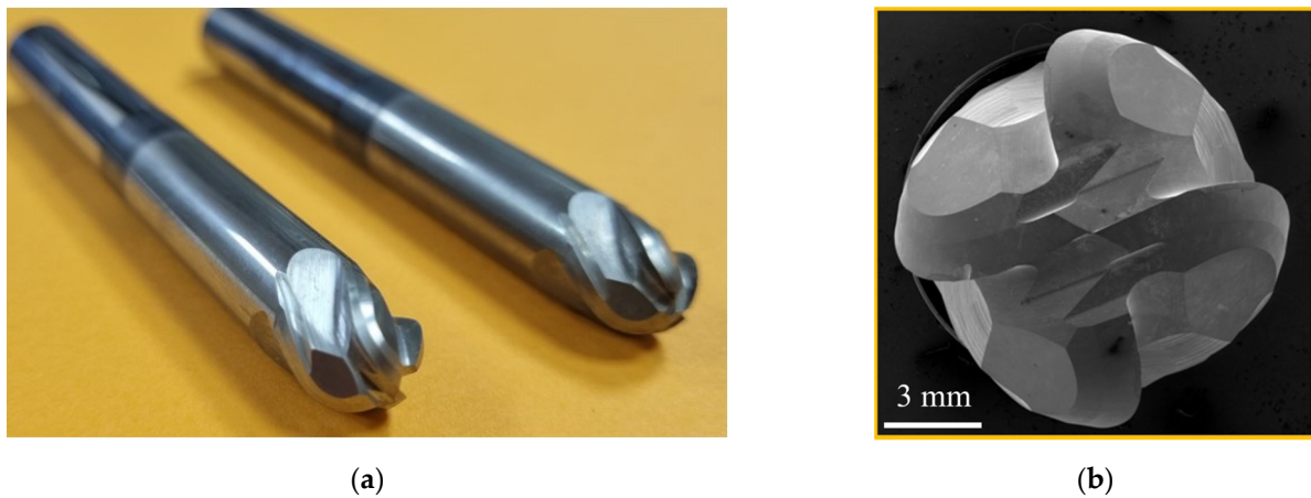
Figure 5. General view (a) and end nose design (b) of carbide ball-end mills used for coating and subsequent testing in cutting Inconel 718 alloy.
