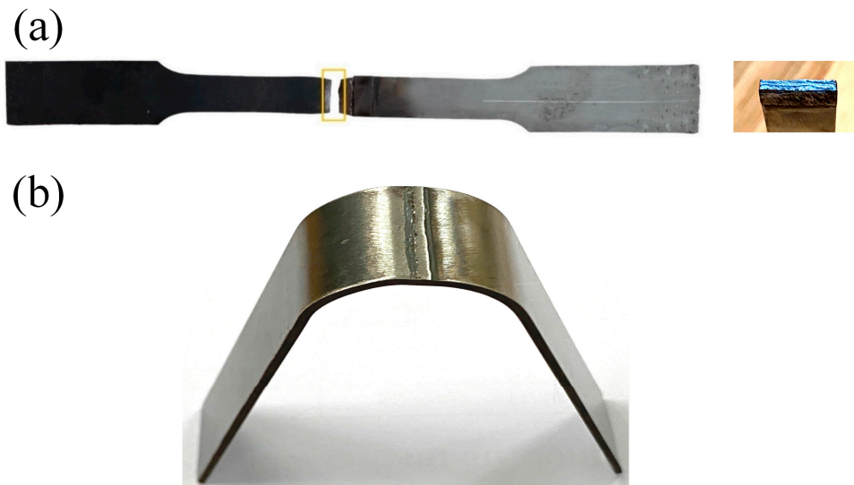
Figure 9. Sample after test: (a) tensile test, and (b) bending test.
