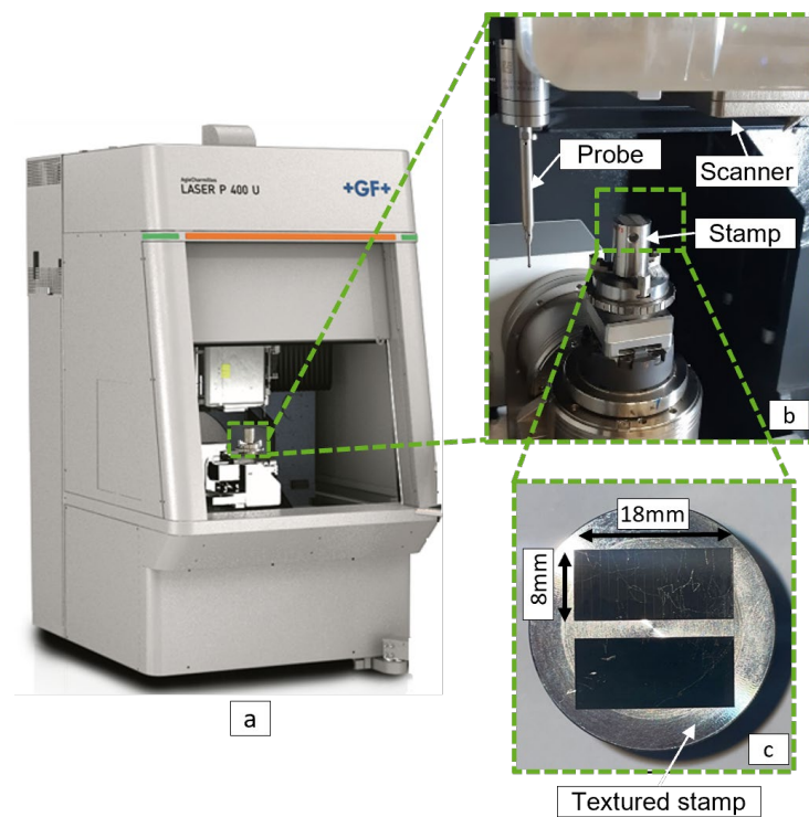
Figure 2. (a) Five-axis laser machine; (b) Positioning of stamp; and (c) Dimensions of laser-textured stamp.
