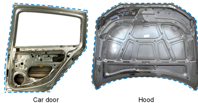
Figure 1. Example components with hemmed outer edges.
