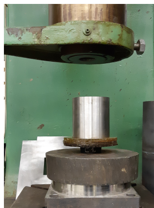
Figure 3. Cutting setup on the Hidroma Press.
