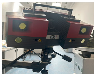
Figure 2. The applied GOM Atos scanner.
