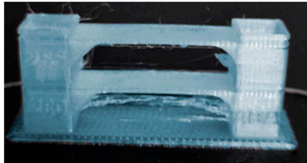
Figure 5. Printed temperature tower.
