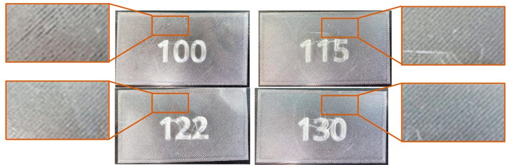
**Figure 10.** Samples with different flow values.
