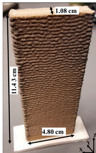
Figure 1. Image of the as-built rectangular WE43 magnesium alloy specimen produced by LPDED. Z-direction represents build direction.
