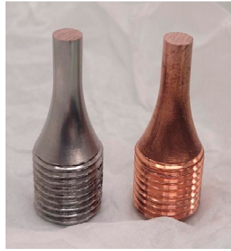
Figure 25. Thermally exposed fatigue specimen TE6.
