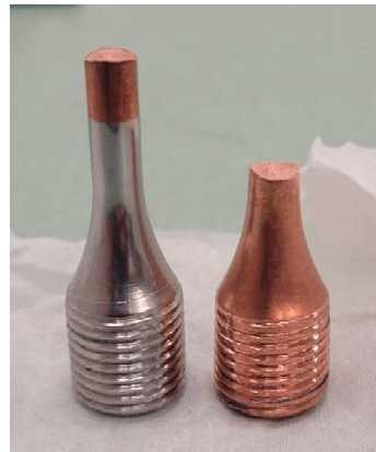
Figure 21. Thermally exposed fatigue specimen TE1.
