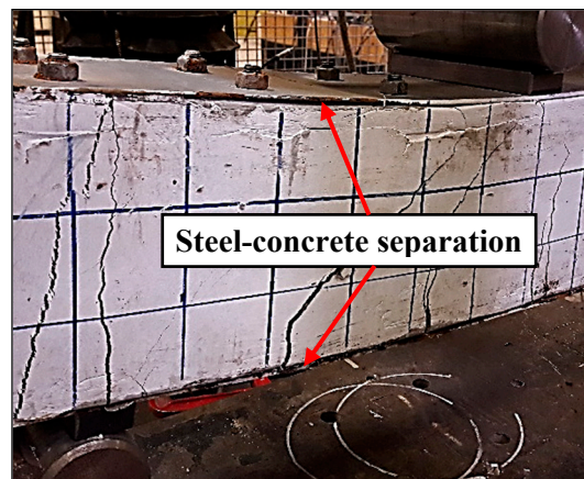
Figure 10. Steel–concrete separation in Rub-B specimen.
