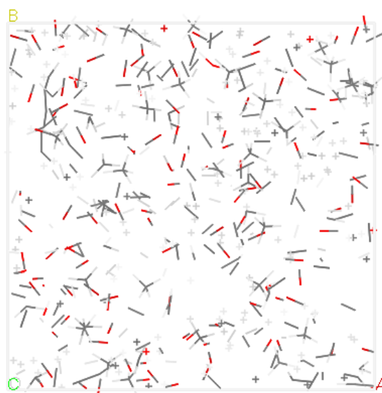
Figure 6. Model of 1000 atoms, 100% cured at 1250 K after 1.5 ns.
