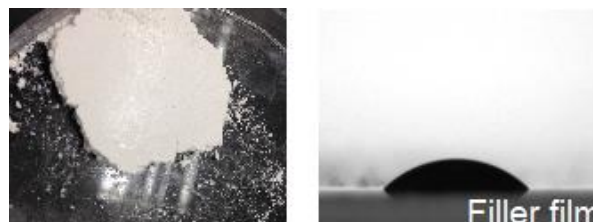
Figure 3. Contact angle measurement on a thin film of nanoparticles. On the left, a film obtained by compression of the particles, and on the right, a water drop on the surface of the film.
