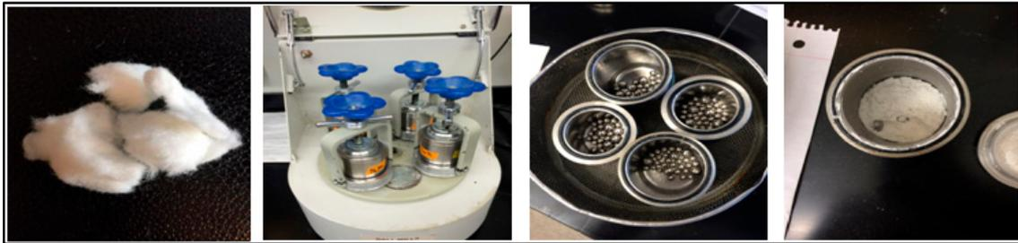
**Figure 1.** The cellulose pulp, ball mill, steel jars and balls, and powdered cellulose (left to right).
