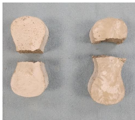
Figure 12. Brittle failure of unreinforced mortar mix, base material (MC) (left) and ductile cup and cone fracture for reinforced mortar, MFS (right).
