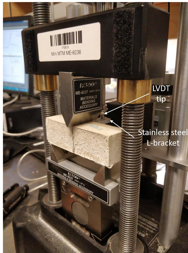
Figure 8. Arrangement of the displacement measuring set up for beams.
