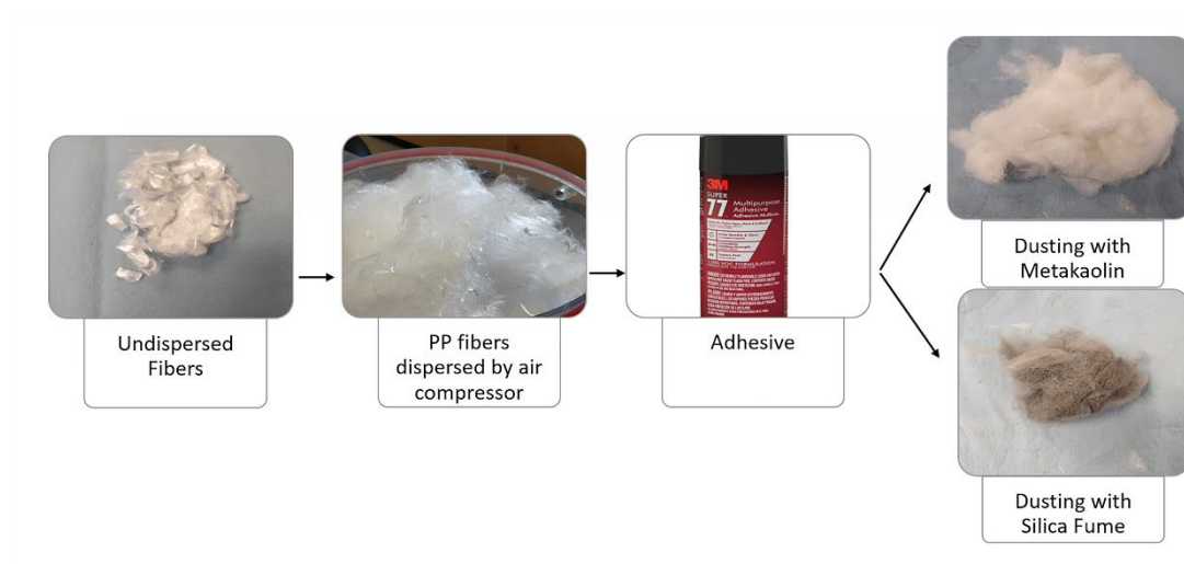
Figure 3. Chart showing the process of fiber preparation.
