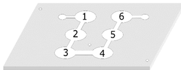
Figure 6. Silicon mold (corresponding to point 3 in Figure 2), which allows for the production of six discs of 20 mm diameter per 1.5 mm thickness.
