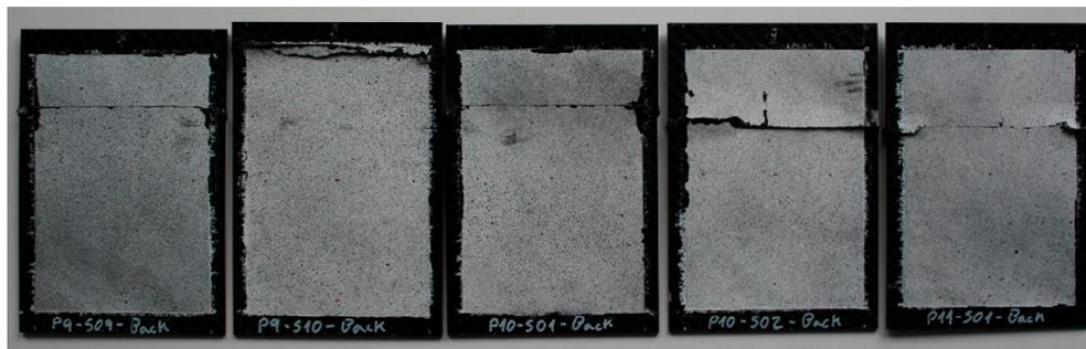
Figure 8. Front side of tested specimens using New CAI device.
