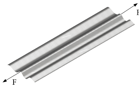
Figure 4. Wrinkling of initially planar unidirectional (UD) ply due to shear buckling in off-axis tensile test.
