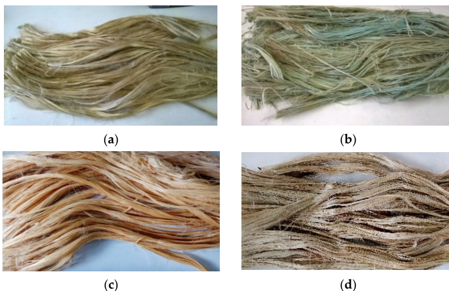
Figure 2. Appearance of (a) Raw, (b) RT, (c) FT, and (d) WT treated jute fibers.
